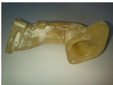
Gambar 2. Intake Manifold Komposit Serat Nanas
