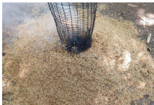
Figure 1. The production of biochar by a simple pyrolyzer.
