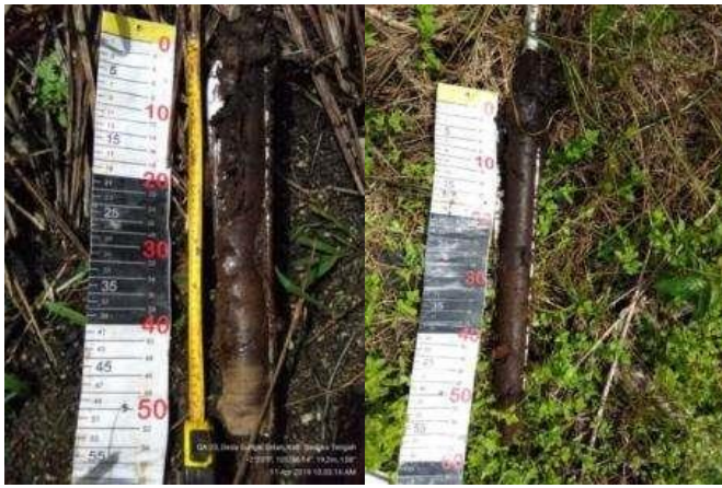
Figure 4. Cross-sectional view of peat soil at various depths in Central Bangka Regency
