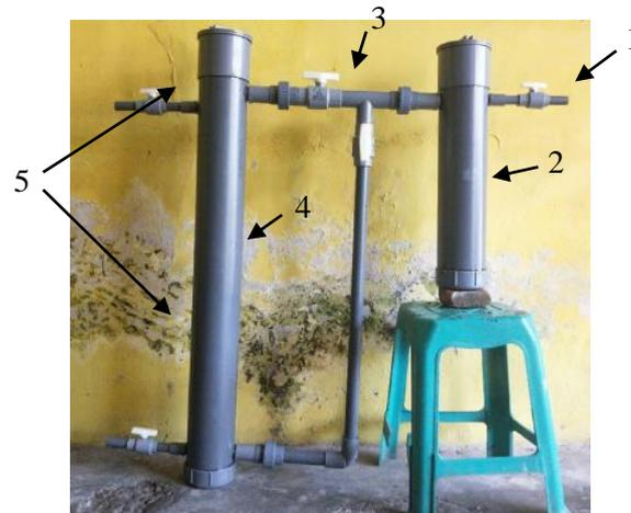
Gambar 1. Desain *simple water filtration*
