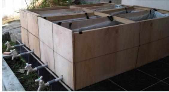
**Gambar 1. Reaktor SSF-Wetland**
