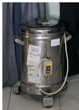
Figure 5. Spinner is being introduced to drain oil from deep-fried peanuts
