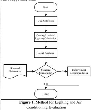
Data collection is conducted through observation, interviews, and measurements. The next stage involves the calculation of lighting and cooling loads. Lighting calculations aim to determine the quantity and type of lamps needed, while cooling load calculations are performed to determine the required capacity of the air conditioning unit. Lighting calculations utilize the Lumen method (Badan Standardisasi Nasional, 2011) as shown in the following equation:
