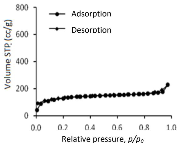
**Figure 3.** Adsorption-desorption N<sub>2</sub> of mesoporous silica synthesized by sonochemical method
