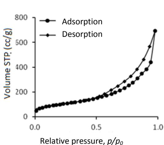
**Figure 2.** Adsorption-desorption N<sub>2</sub> of mesoporous silica synthesized by hydrothermal method
