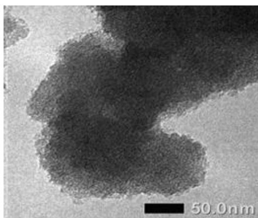
**Figure 5.** TEM micrograph of mesoporous silica synthesized by sonochemical method
