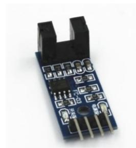
Gambar 2. *Sensor Optocoupler*
