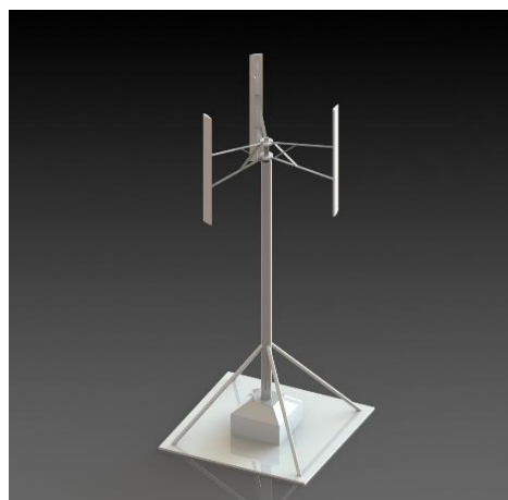
Figure 3. Vertically Axis Hybrid Wind Turbine Construction
