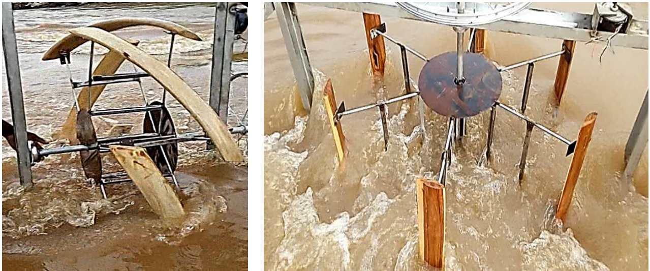
Figure 5. Evaluation of the hydrokinetic geometries in a controlled riverine environment
