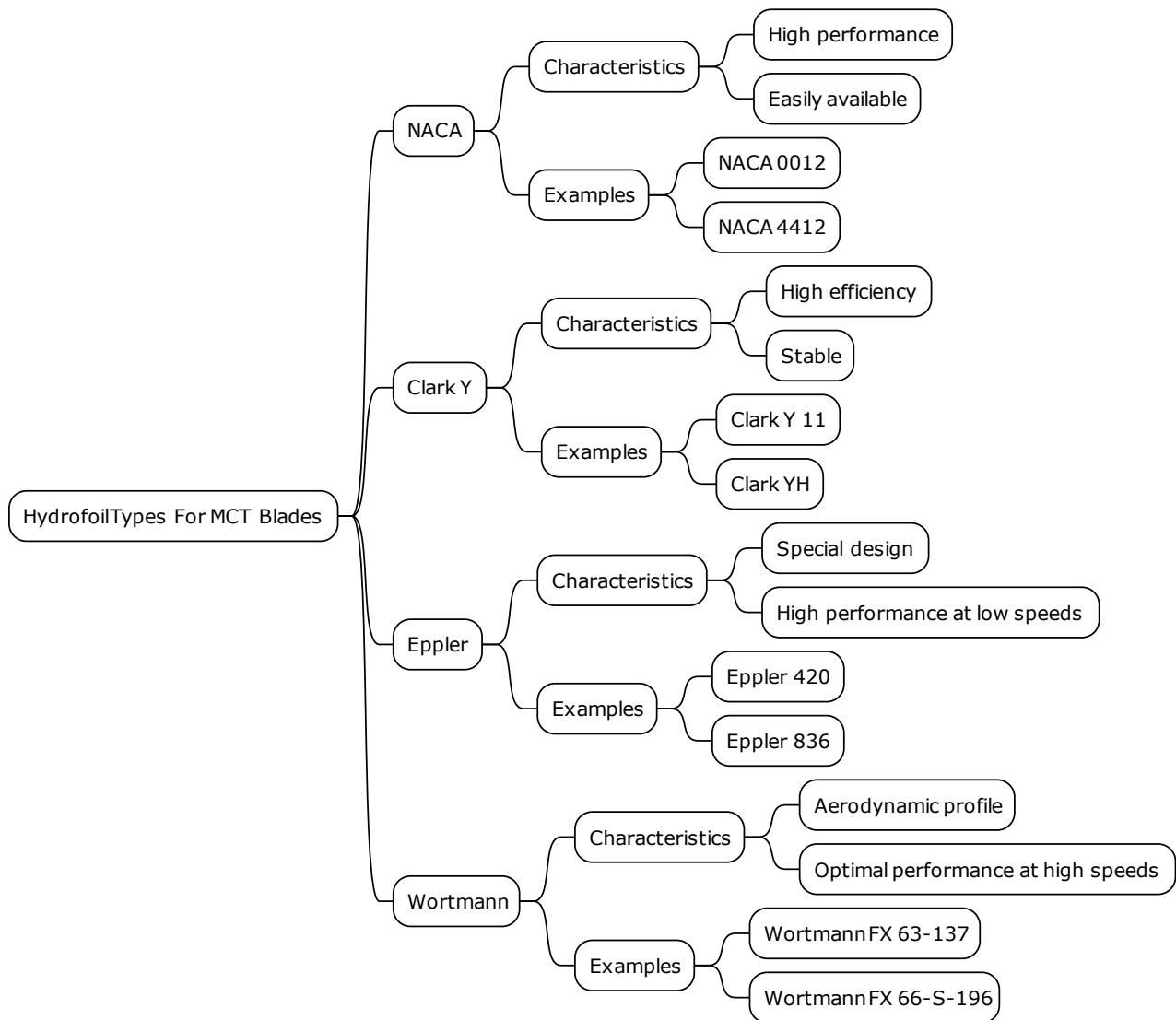
Figure 7. Various types of hydrofoils for OCTs
