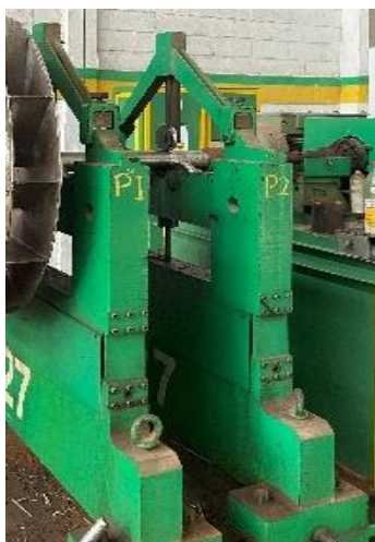
Figure 4. Planes 1 and 2 on the balancing machine
