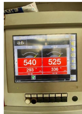
Figure 6. Balancing machine monitor
