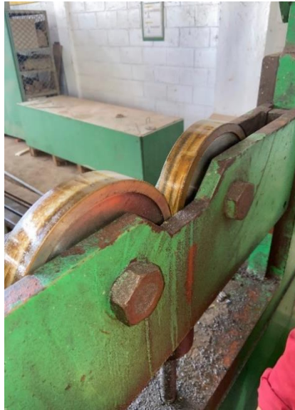
Figure 9. Bearings of balancing machine
