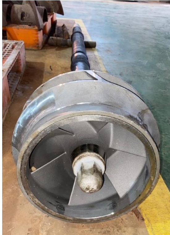
Figure 8. Single – suction closed type impeller
