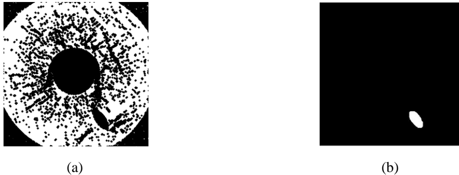
Figure 8. (a) CT Slice 400th after segmentation, and (b) CT Slice 400th after morphological operation
