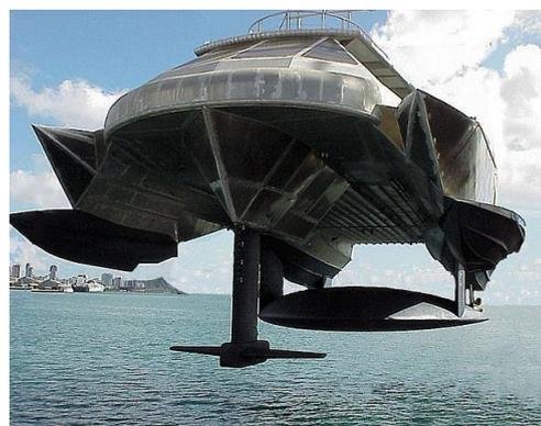
**Figure 2.** Lifting body of the ship hull [23]
