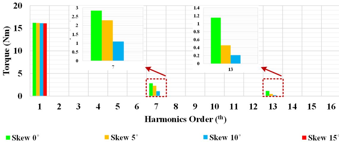
Figure 6. Torque harmonics bar curve with stator skew angle variations
