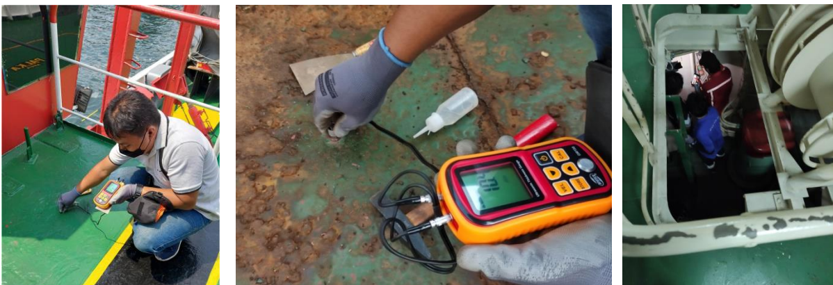
Figure 8. UT inspection on Baruna Jaya IV Vessel
