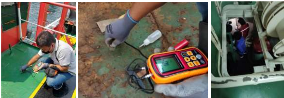
Figure 7. UT Inspection on Baruna Jaya IV Vessel
