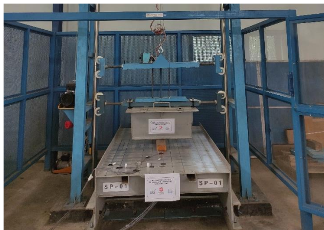
Figure 3. Experimental study on side shell structure of fast patrol boat
