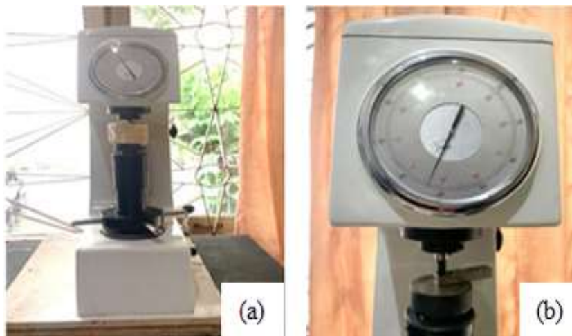
Figure 4. (a) Rockwell hardness tester machine (b) Testing specimen
