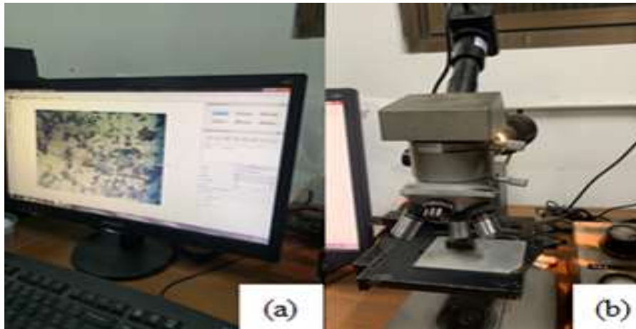
Figure 5. Macrostructural analysis tool: (a) PC (b) Metallography microscope
