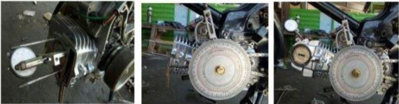
Figure 1. Engine compression ratio adjustment
