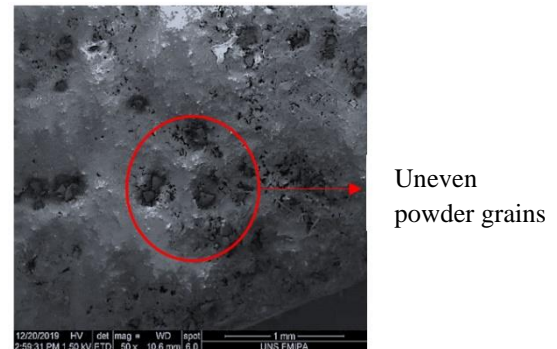
Figure 5. SEM surface of epoxy with aluminum powder filler
