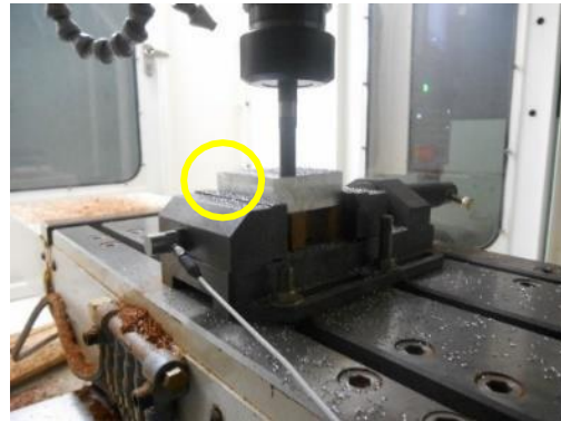
Figure 2. Piezoelectric Accelerometer Sensor Placement
