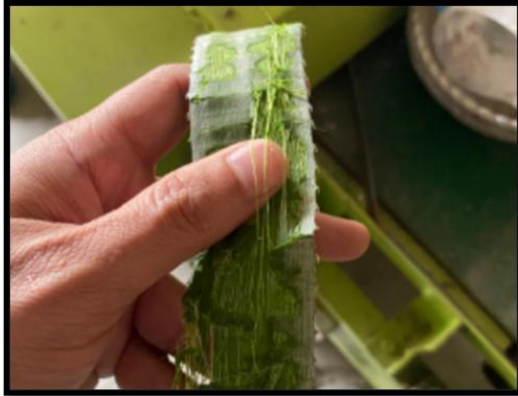
Figure 5. Clean and continuous PALF extracted through the mechanical process
