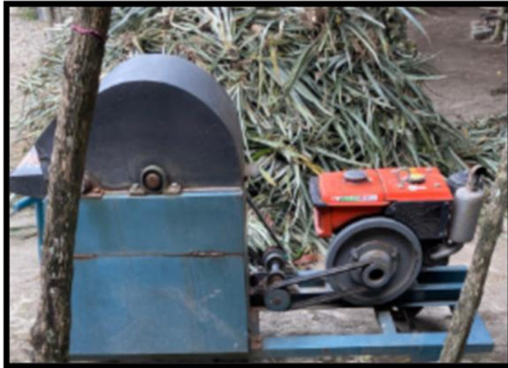
Figure 3. The mechanical decorticator machine is used for fiber extraction
