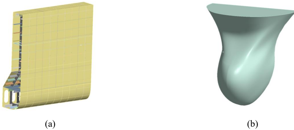
Figure 3. Modeled design for collision analysis in this study: (a) The struck ship (lower section of double hull) and (b) The striking ship (bulbous bow)
