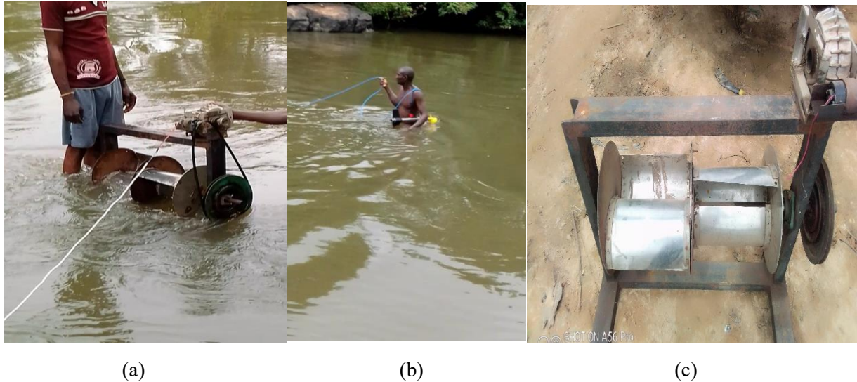
Figure 8. (a) Experimental test activities in River Ogun, (b) Gauging activities in the river, and (c) The double-stage Savonius test turbine
