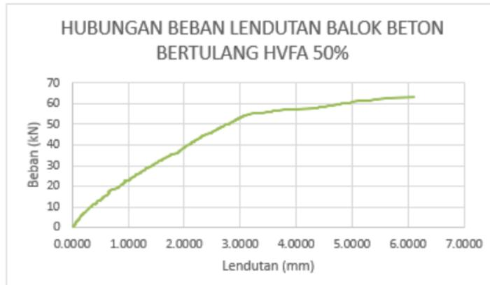
Gambar 3. Grafik Beban-Lendutan Balok Beton Bertulang Beton HVFA-SCC 50%
