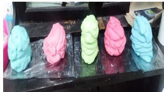
Figure 1. Micro wax-based plasticine (left), petroleum jelly based plasticine (right)
