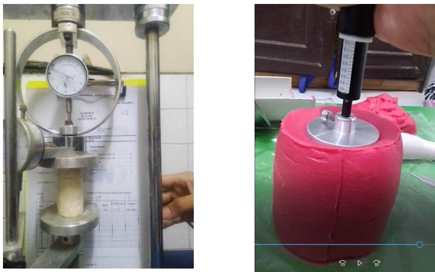
Figure 3. Unconfined compression strength test (left) and hand penetrometer test (right)
