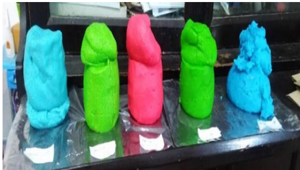
Figure 1. Micro wax-based plasticine (left), petroleum jelly based plasticine (right)
