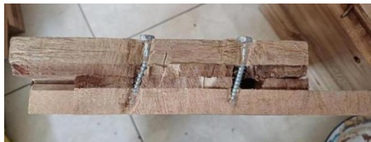
Gambar. 6 Mode Keruntuhan Lag Screw 1
