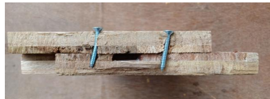
Gambar. 7 Mode Keruntuhan Tapping Screw 2
