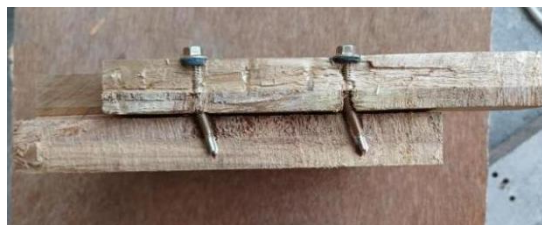
Gambar. 8 Mode Keruntuhan Drilling Screw 1
