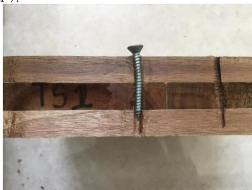
Gambar 6. Mode keruntuhan *tapping screw*
