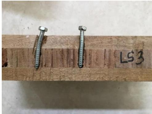
Gambar 7. Mode keruntuhan *lag screw*
