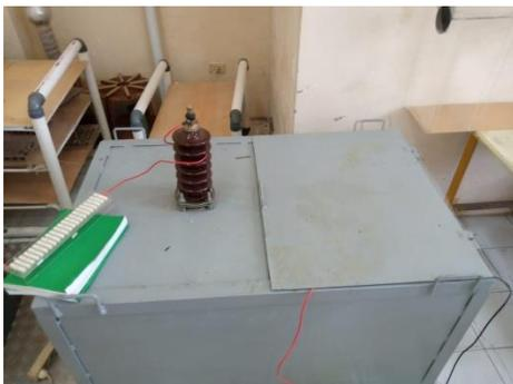
Gambar 2. Model Tangki Transformator
