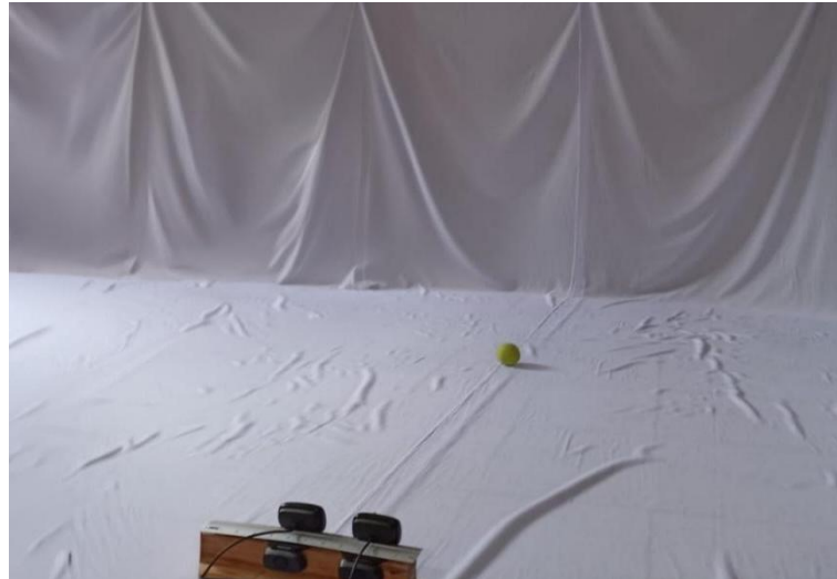
Figure 1. Configuration of a stereo camera with a tennis ball for collecting training and validation images.
