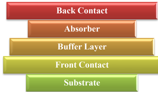
Figure 12. Standard structure of solar cells
