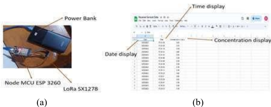
Figure 4. (a) Fiber optic sensor data receiver (b) sensor data display and storage
