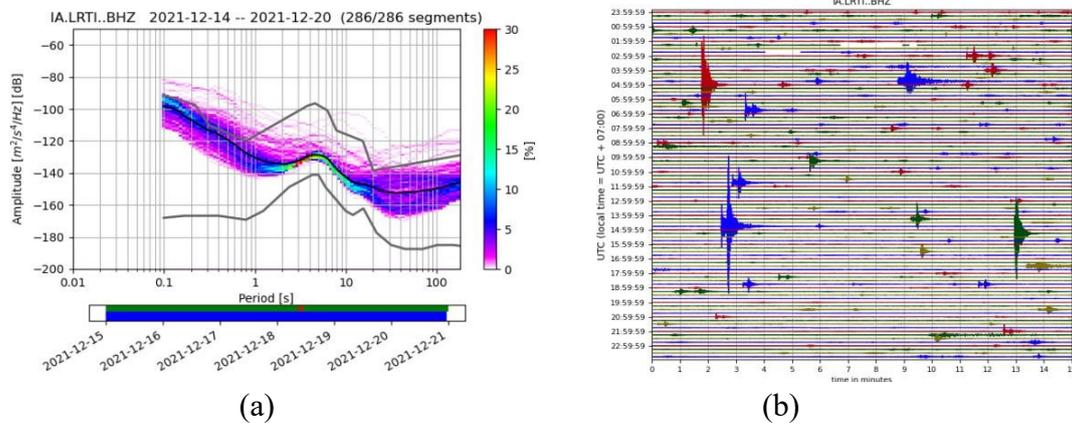
**Figure 8.** Probability Spectral Density Function of aftershocks (a) Amplitudeaftershock (b) Noise seismogram (Hakim et al., 2022)
