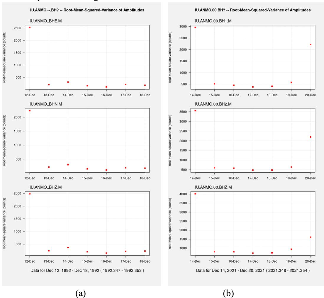
**Figure 7.** The RMS distribution value is obtained by the Probability Spectral Density Function (a) Amplitude of the aftershocks of 12 December 1992; (b) Aftershock amplitude of 14 December 2021
