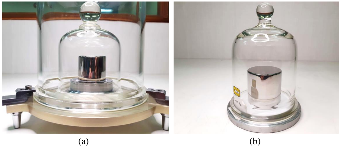
Figure 1. (a) Pt-Ir national standard, and (b) E 0 class mass work standard no. 74.
