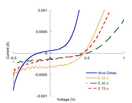
Figure 4. Characterization of current-voltage (I-V) from time variation Cu on TiO<sub>2</sub> trough electroplating method
