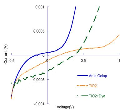
Figure 3. Characterization of current-voltage (I-V) from TiO<sub>2</sub> and TiO<sub>2</sub>-dye
