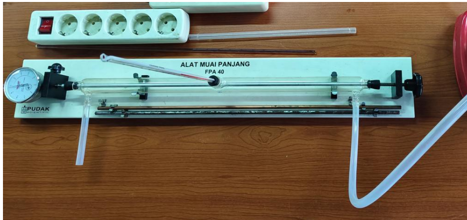
Figure 2. The hot steam enters from a single point on the right end, whereas condensed at the opposite end.
