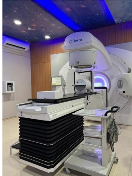
Figure 4 Setting for QA planning using Octavius phantom
