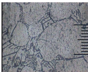
Figure 7. Photographs of microstructure with variations of 4% Mg addition at 200 times magnification
