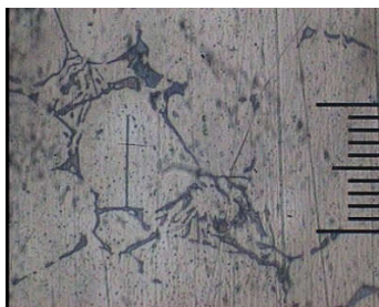
Figure 6. Photographs of microstructure with variations of the addition of 3% Mg at 200 times magnification
