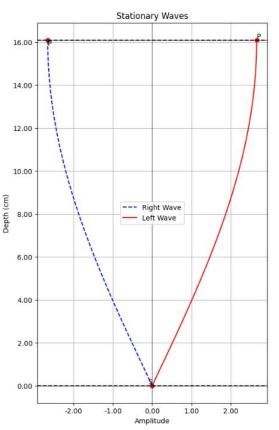
Figure 5. Wave at the First Resonance of a Closed Organ Pipe
