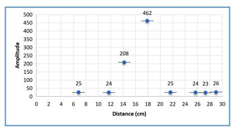
Figure 4. Graph of the Relationship Between Distance and Amplitude: Identification of Resonance Points
