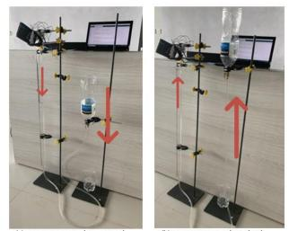
(a) Water Reservoir Lowered (b) Water Reservoir Raised **Figure 2.** Illustrates the process of adjusting the water level to influence the resonance in the tube.
