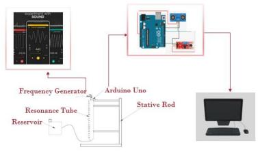
Figure 1. Sound Resonance Experiment Setup Diagram.
