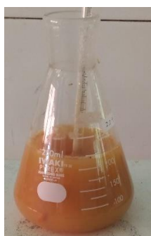
Figure 1. The formation of the brown precipitate in the reaction mixture consisting of 50 ml of 0.1 M \text{SnCl}_4 , 50 ml of Garcinia mangostana L fruit peels extract with a mass of 2.5 g and 100 ml of 0.1 M NaOH.
