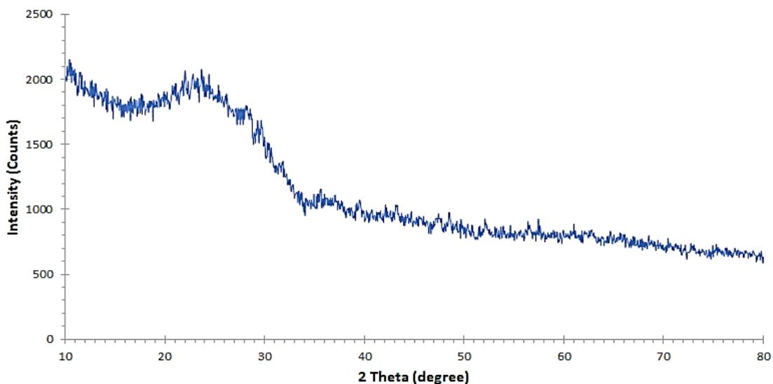
**Figure 4.** The amorphous phase of a glass bottle.
