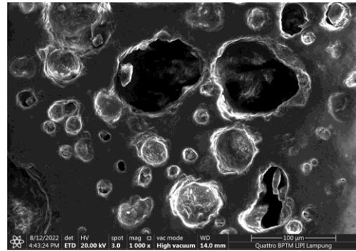
Figure 6. The surface topography of foam glass-ceramics.
