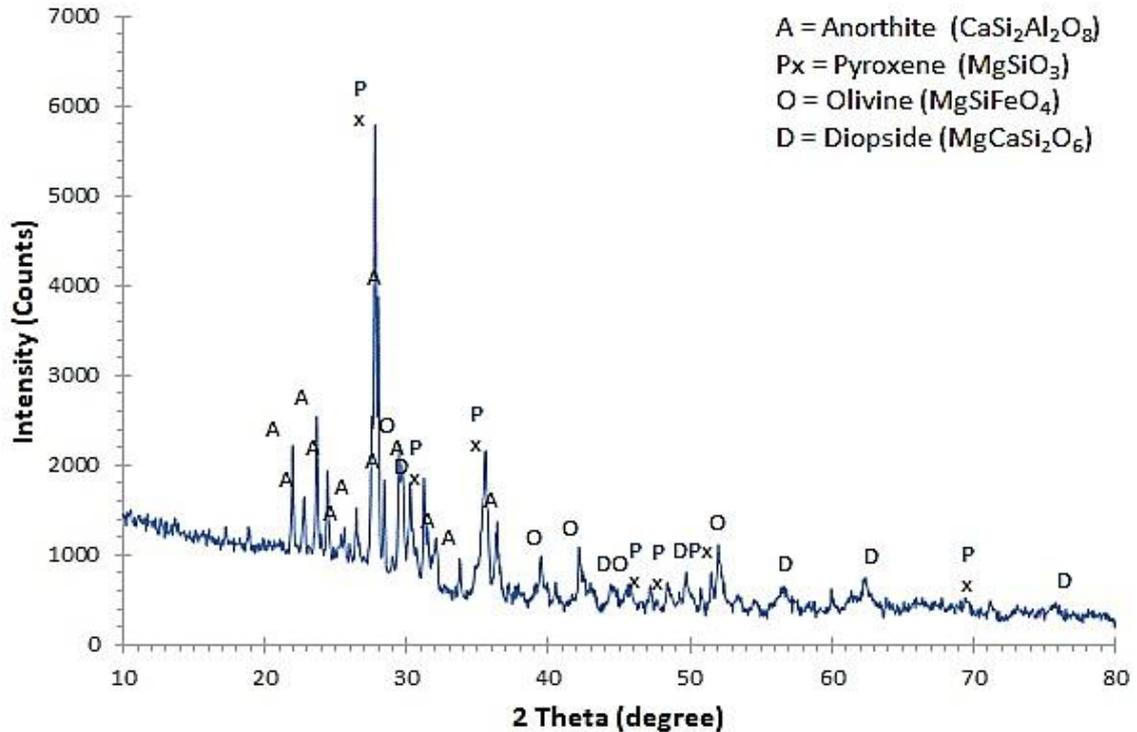
**Figure 1.** Crystal phase of raw basalt.
