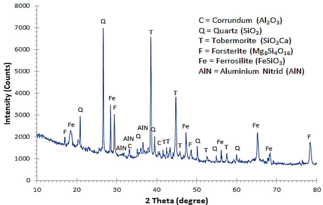
Figure 3. Crystal Phase of Aluminum Dross
