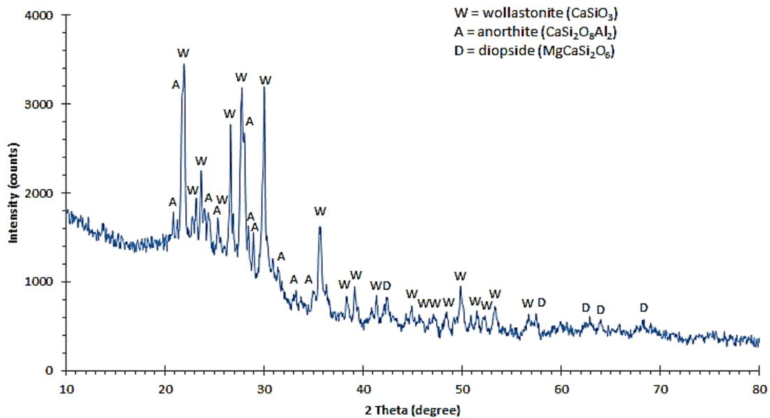
Figure 5. The crystal phase of foam glass-ceramics.
