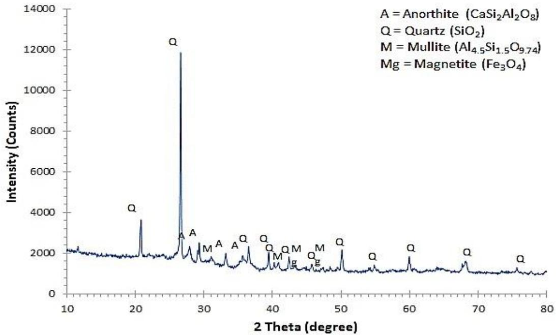
Figure 2. Crystal phase of fly ash
