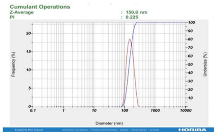
Figure 6. Results of particle distribution with PSA on nanoparticles
