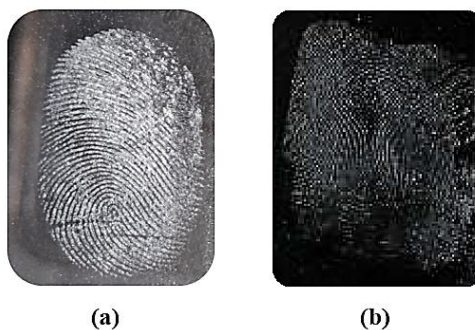
Figure 8. Comparison of latent fingerprint visualization on a glass slide: (a) ZnO nanoparticle biosynthesis powder from durian peel, (b) HI-FI Volcano Latent Print Powder
