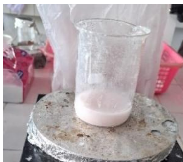
Figure 2. Homogenization process of silica and cochineal solution using a magnetic stirrer.
