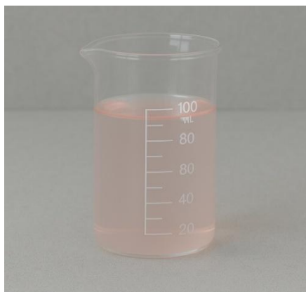
Figure 1. Filtrate Resulting from the Extraction of Cochineal Insect Powder
