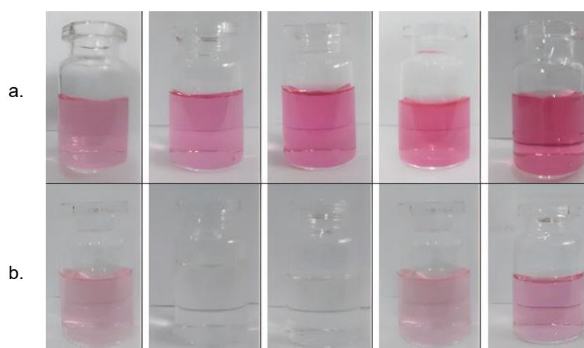
Figure 7. Colour change of Remazol red test solution at concentrations of 10, 20, 30, 40, and 50 mg/L, a) before coagulation and b) after coagulation.
