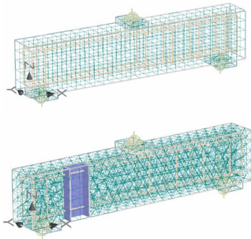
Fig.6 FE meshing on beam
