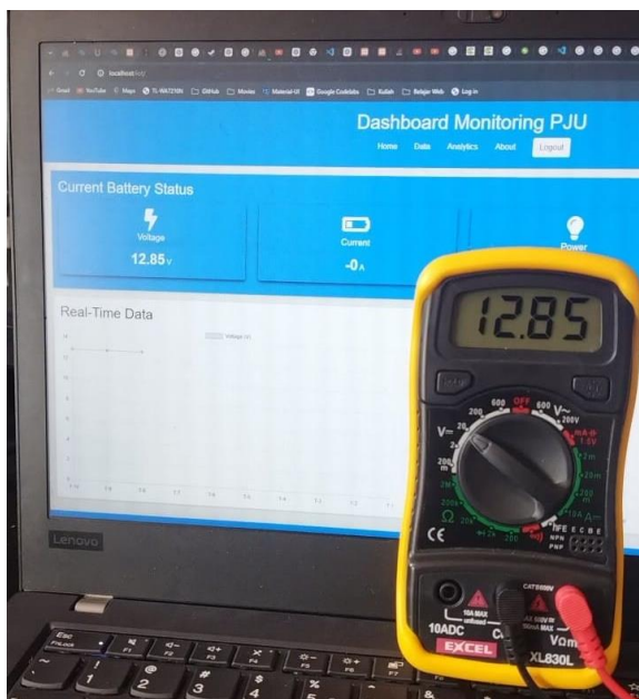
Fig. 13. Accuracy Test of INA219 Voltage Measurement Sensor
