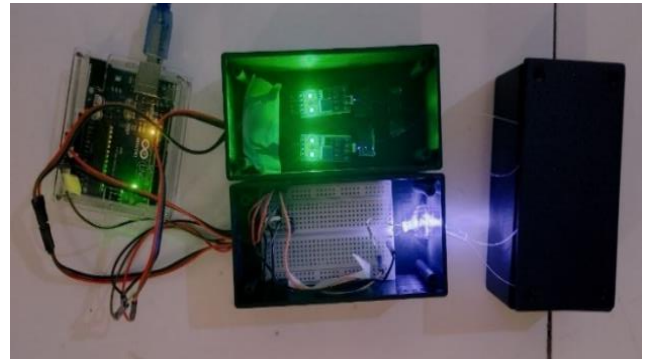
Fig. 2. Light travels through the reference and modulated fiber optic (macrobending) in the black box
