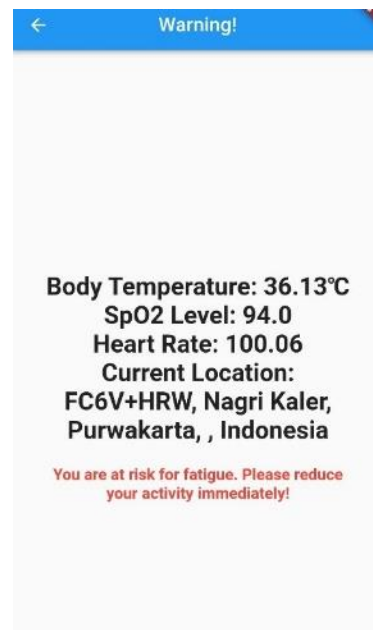
Fig. 13. The detailed information on warning page of the Smart Ring application
